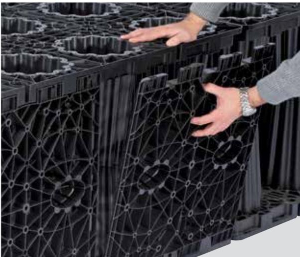
The outsides of the tank must be covered with side panels that click into place. These are inserted into the openings provided in the tank body elements. The side panels create a perimeter for the entire system offering a consistent surface for the geomembrane or geotextile. If needed, a pipe connection point can be cut out along the cutting guides in locations provided. Side panels have cutting guides for the connection of plastic pipes.
